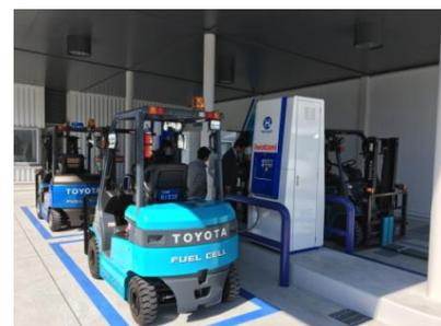
Hydrogen fuel cell powered forklifts
