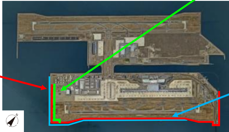
Raising of south cut-off wall
