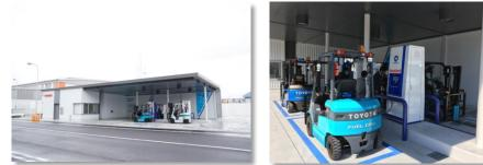
Hydrogen fuel cell powered forklifts
