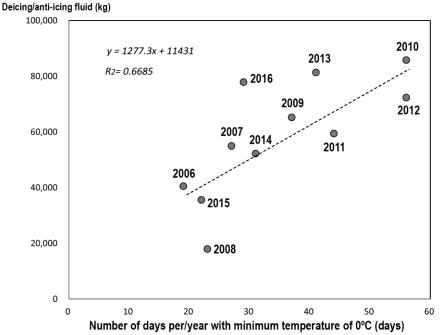
Correlation between minimum temperature and use of deicing/anti-icing fluid
