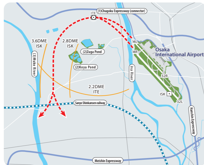
← Red dotted line: Preferential flight paths Orange line: Area of preferential flight paths
