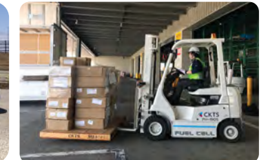
Introduce fuel-cell forklifts
