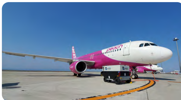
An electrical Ground Power Unit (eGPU)
